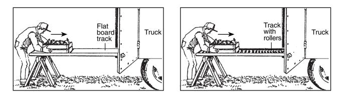
The person using the track with the rollers uses less energy to load the box because the rollers reduce the
