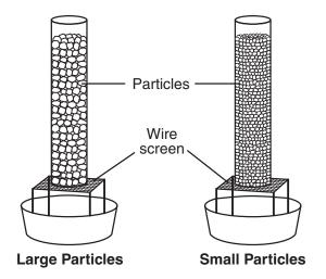
Two identical columns contained equal volumes of different-size particles. The same amount of water was added to the top of each column. A student timed how long it took for the water in each column to reach the wire screen. The data table below shows the results.
